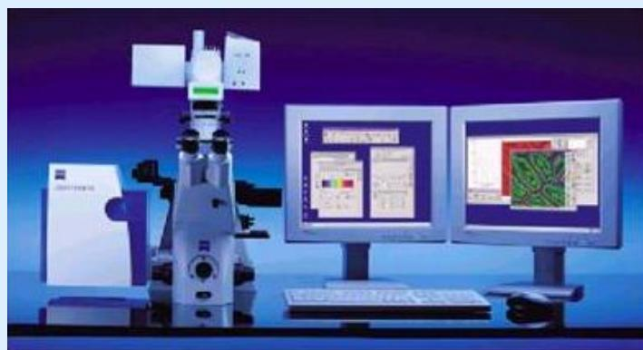
Figure 1: Microscope confocal Zeiss LSM 510
